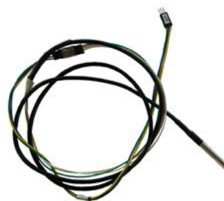
Figure 6. The water temperature sensor used in the study
