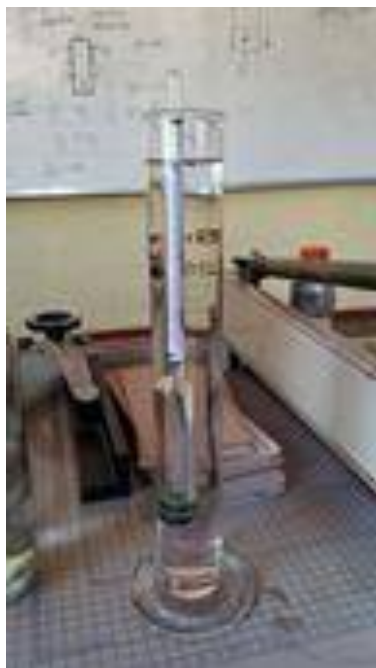
Figure 4. Concentration of ethanol determination using the hydrometer.
