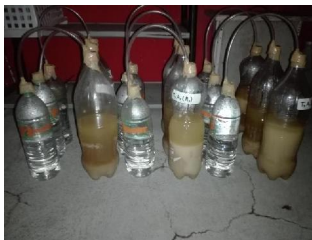
Figure 3. Airlock of the feedstock during the fermentation process.
