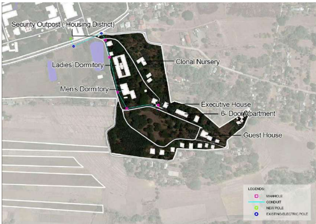
Figure 2-13: Underground Fiber Optics Layout Zone 4
