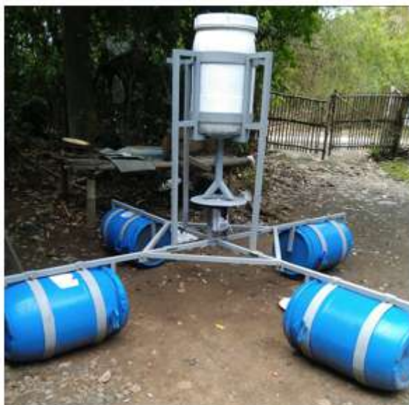
Figure 25. The fabricated Automatic Tilapia Feeder
