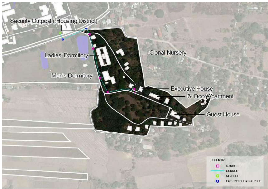
Figure 2-13: Underground Fiber Optics Layout Zone 4
