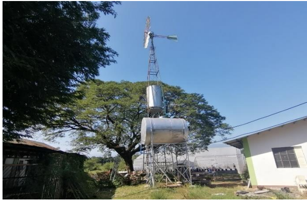
Figure 6.5.4k. Windmill-driven pumps with an elevated water tank.
