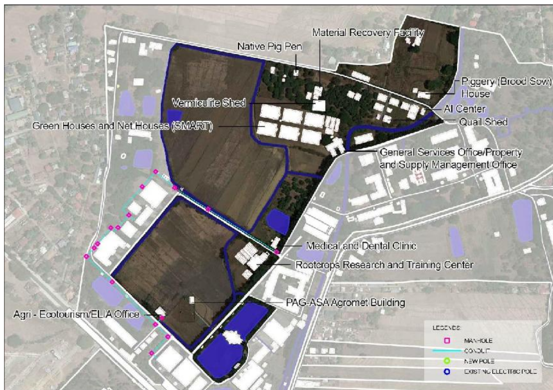
Figure 2-10: Underground Fiber Optics Layout Zone 1
