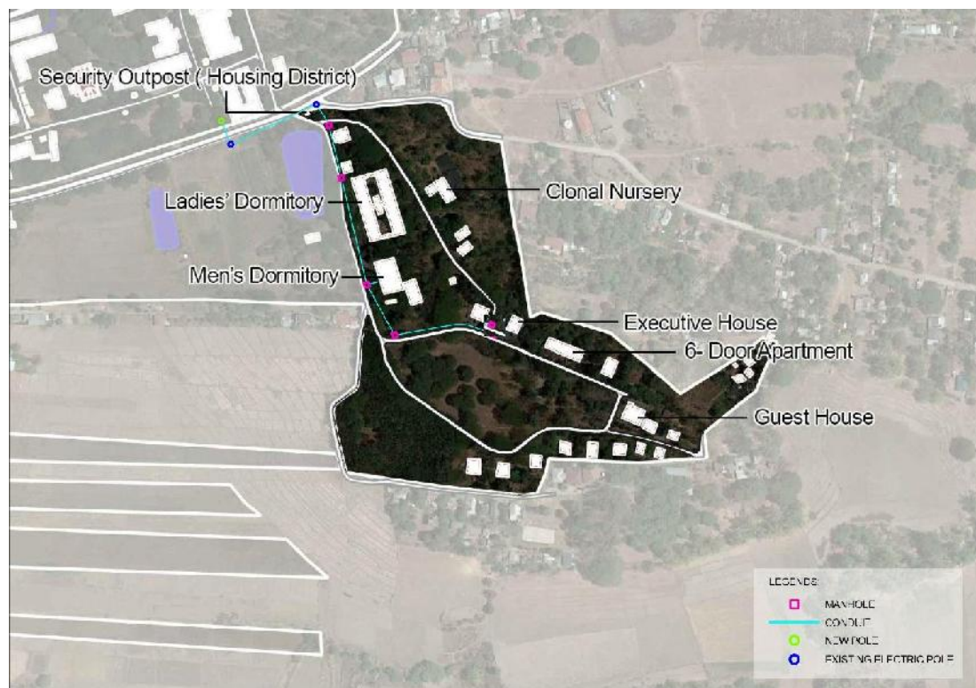
Figure 2-13: Underground Fiber Optics Layout Zone 4
